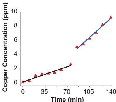
*Note.* Each Moscow Mule solution initially was sparged with nitrogen gas to remove atmospheric oxygen and then placed in the copper mug under a nitrogen atmosphere. At 75 min, the solution was sparged with atmospheric gas for 15 min to replenish dissolved oxygen. Linear fits of the oxygen-free (black) and oxygen-reintroduced (blue) regions are shown.
