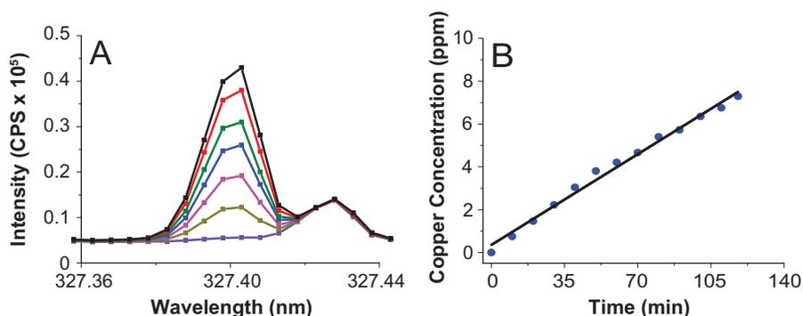
*Note.* A) ICP-AES of copper from a Moscow Mule solution held within a copper mug at 0 min (purple), 20 min (dark yellow), 40 min (magenta), 60 min (blue), 80 min (green), 100 min (red), and 120 min (black). B) Copper concentration as a function of time for a Moscow Mule solution held within a copper mug. The copper concentration (blue circles) as a function of time was fit with a linear trendline (black). CPS = counts per second.
