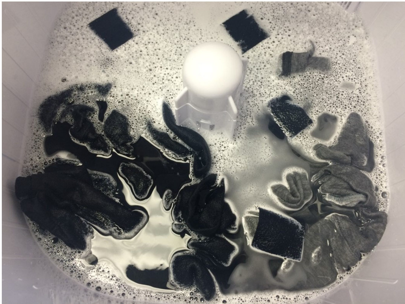
Figure: Simulated laundry load including water, detergent, clothing, and four cotton swatches
